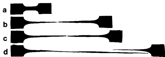
Figure 2 Silhouettes of Sn-Pb tensile specimens tested to failure at various constant cross-head velocities: (a) undeformed, (b) 0.2 \text{ cm min}^{-1} , (c) 0.1 \text{ cm min}^{-1} , (d) 0.05 \text{ cm min}^{-1} .
