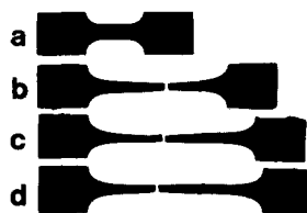
Figure 3 Silhouettes of Sn-Pb-Ag tensile specimens tested to failure at various constant cross-head velocities. (a) undeformed, (b) 0.2 \text{ cm min}^{-1} , (c) 0.1 \text{ cm min}^{-1} , (d) 0.05 \text{ cm min}^{-1} .
